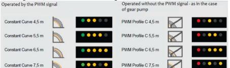
To see how to set the pump, briefly press the button  $\mathbf{\hat{N}}$ . For the duration of 3 seconds the pump will display one of the
